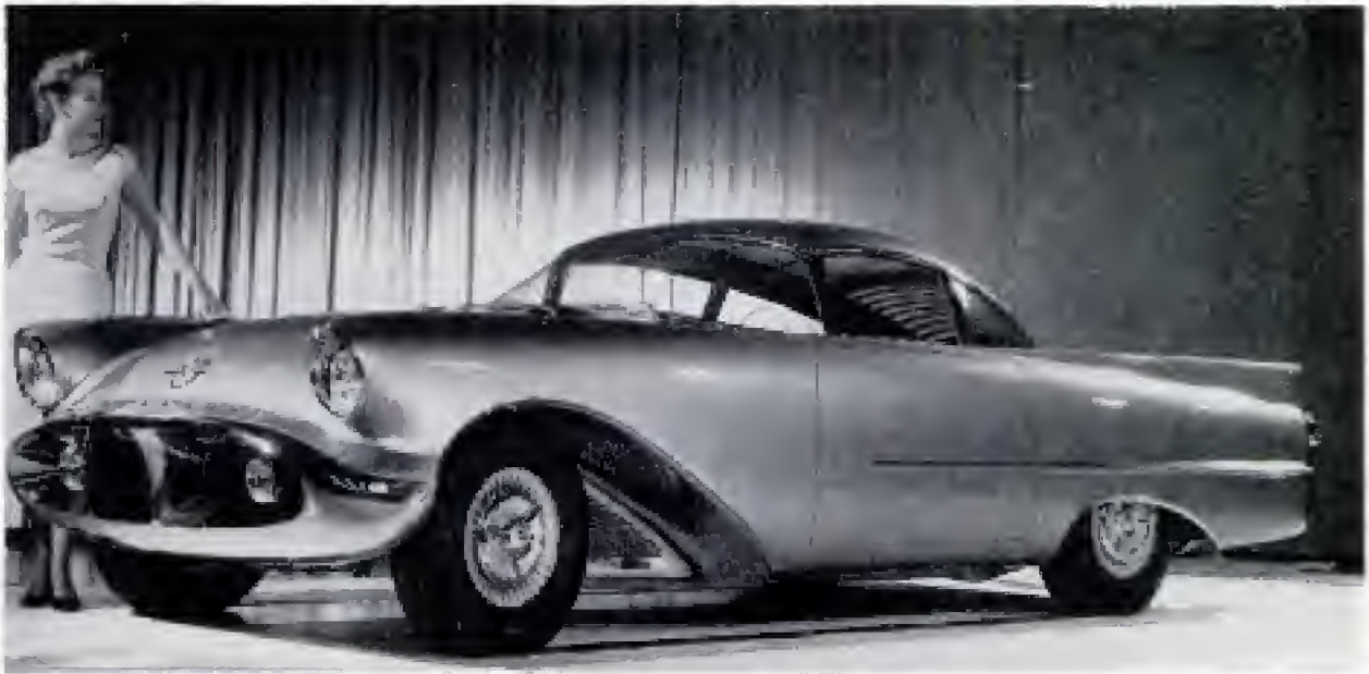
OLDSMOBILE calls its model the Cutlass. Recessed headlights, high tail fins and a bubble-like top give it a futuristic look. Front-wheel housings are perforated to exhaust engine heat. See page 91 for Buick's Wildcat
